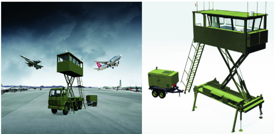
Fig. 1 and 2. Portable air traffic control tower.
